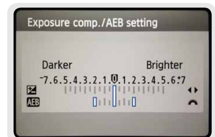
Canon Rebel T2i/550D LCD showing AEB with +/- 2 EV increments selected
